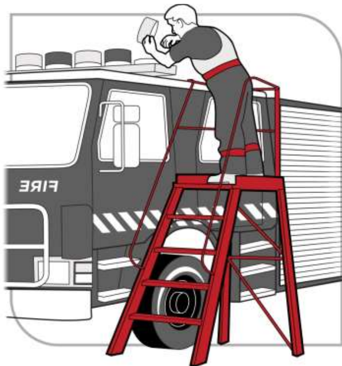
Figure 1 A step platform can provide a stable work surface
